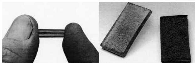
Figure 16. Plasma fragmentation of two JA2 stripes in an “open” experiment.
