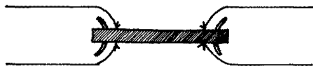
Figure 83. Cross-matched time fuse with buckets tied over ends.
